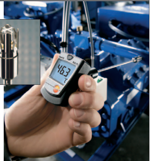
Monitoring surface temperature in refrigeration systems
