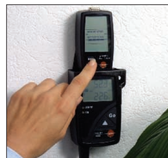
Collect data on-site with the testo 580 data collector, download and analyse on PC/Notebook.
