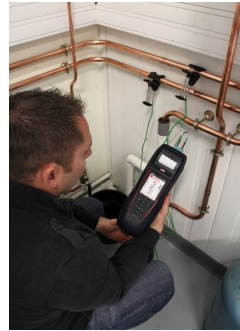
DHW network temperature
