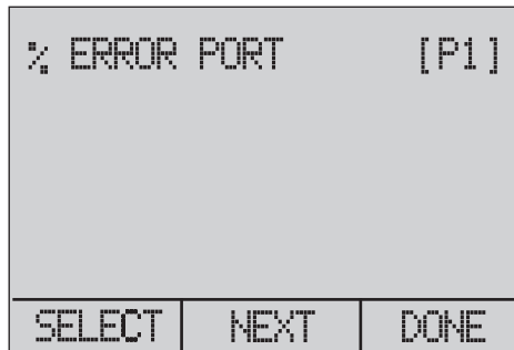
Figure 29. Port Setting Screen
