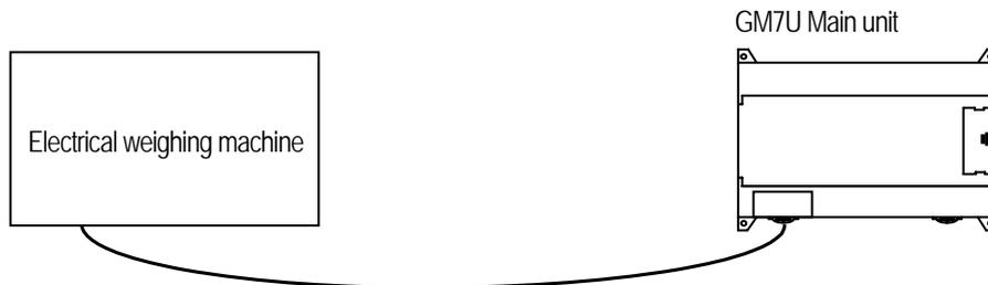
For No Protocol Communication, one of following end condition is designated. One is the size of the received data, and the other is the received data setting that is the same with pre-defined data.
