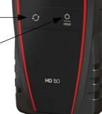
Auto shut-off: the instrument switches off if not used during 20 minutes.
