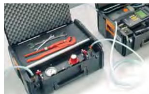
Standard testing pressure compensation with feeding unit
