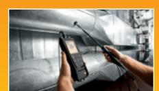
When taking duct measurements, the testo 480 can measure the flow within the duct and complete HVAC grid measurements so the system can be adjusted optimally.
