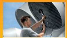
When measuring at air outlets, the 480 can check whether a system is optimally configured and balanced, allowing the HVAC professional to take any necessary corrective measures and improve the indoor air conditioning quickly and easily.
