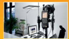
A full line of probes are available for measuring comfort level and indoor air quality for a wide variety of different circumstances. A tripod is also available for use with the 480 for workplace evaluation.
