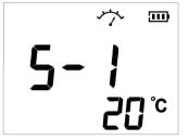
Fig. 11 Fig. 12 Suggestions for selection of calibrating gas concentration: for maintenance inspection, the value of calibrated concentration can be around 220ppm; for low concentration alarm, the value of calibrated concentration can be around 53ppm. The inspection of professional institute can refer to the requirements of inspection rules JJG-915-2008 to choose 700ppm as the calibrated concentration value
