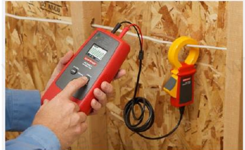
Induce signal with the signal clamp when there is no bare conductor.
