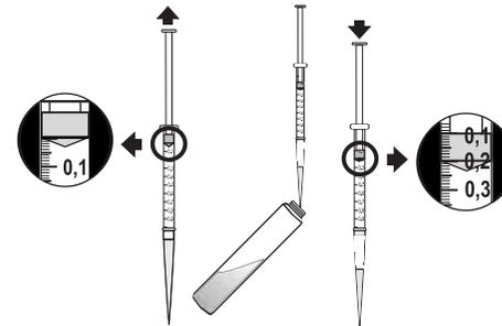
**Note:** to measure exactly 0.2 mL of sample with the syringe, push the plunger completely into the syringe and insert the tip into sample. Pull the plunger out until the lower edge of the seal is on the 0.0 mL mark of the syringe. Insert the syringe into the vial and push the sample out until the lower edge of the seal is on the 0.2 mL mark.
