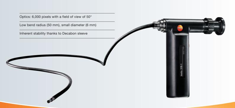
The fiberscope testo 319 allows an easy visual check of difficult-to-access places such as air conditioning ducts, ventilation systems, machines and engines etc. Diagnoses such as corrosion, abrasion, the condition of weld joints, loose parts and much more can be made very early, quickly and easily.
