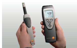
testo 625 with radio handle and radio module
