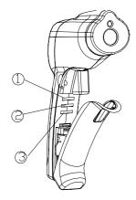
To set values for the High Alarm (HAL), Low Alarm (LAL) and Emissivity (EMS), firstly active the display by pulling the trigger or pressing the MODE button, then press the MODE button until the appropriate code appears in the lower left corner of the display, press the UP and down buttons to adjust the desired values.
