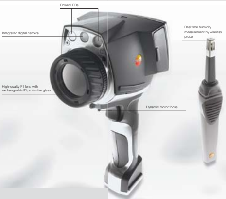
Easy to change wide angle and telephoto lenses for a wide range of applications. The IR protective glass protects the lens from dust and scratches. Easy joystick operation for navigating through menu and image gallery. Surface moisture can be displayed, identifying potential mould-risk spots. Easy navigation and file creation for effortless data management.
