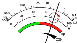
Figure 14: Analogue display indicating ground noise voltage measurement
