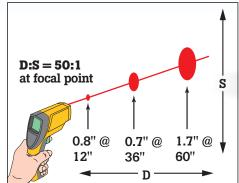
Use the Fluke 68 within 8 m (25 ft.) of the intended target. At greater distances, the measured area will be larger (approximately the distance divided by 50).
