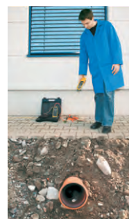
Tracing of underground cables (max. depth 2.5m)
