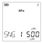
Press "(wm)" key, you can select your desired unit on um to umil, LCD displays as shown below:
