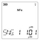
Contact detect head with the test surface vertically and press the detect head lightly, LCD displays a value, for example, 109 μm, and buzzer sounded at this time, LCD displays as shown below:
