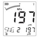
Every time detect head contact the test surface vertically, an reading will be generated with a beep of buzzer. For another measurement, lift the detect head, and repeat the operation above.
