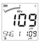
When the second measurement is finished, SNG counter will automatic upgrade to 2. The maximum SNG counter is 15.
