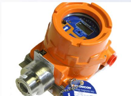
Flamgard Plus is a Flameproof (Ex d), ATEX, IECEx and UL certified flammable gas detector, which uses poison-resistant pellistors to detect explosive levels of hydrocarbons, hydrogen and other flammable gases and vapours, including aviation fuel and leaded petrol vapours.
