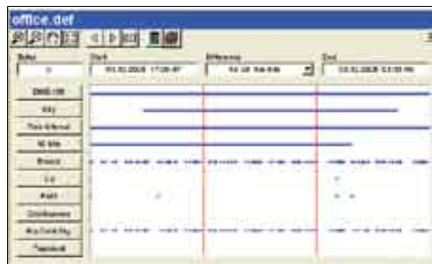
Overview of data for each measurement function. The user can save data transfer time by selecting which data is to be downloaded to the PC.
