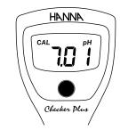
When "7.01" blinks on the display, place the tip of the probe into a pH 4, 7, or 10 buffer solution.
