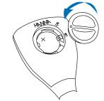
To change the CR2032 Li-ion battery, turn the battery cover located on the back of the meter counterclockwise to unlock. Remove cover and replace with + side facing up.
