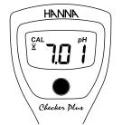
If pH 7 buffer solution is used as the first point the buffer is recognized with the blinking stability indicator.
