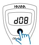
From measurement mode, press and hold the ON/OFF button. The meter will cycle through "OFF," "CAL," then current auto-off setting
