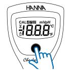
Press the ON/OFF button to turn the meter on. All tags will be displayed.
