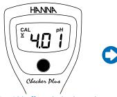
If pH 4 or 10 buffer solution is used as the first point the value of the buffer is recognized and displayed with the blinking stability indicator.
