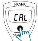
From measurement mode, press and hold the ON/OFF button until "CAL" is displayed.
