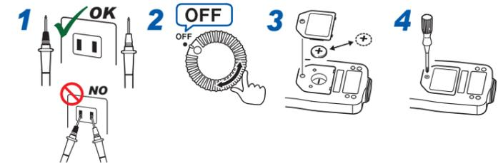
Do not turn the adjustment screw inside the battery case. Doing so will cause the instrument to report abnormal measured values.
