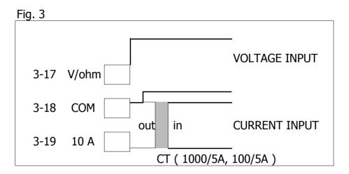
5-8 AC Watt, VA, Whr measurement, current input cooperate with Clamp-On Probe
