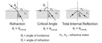
In the MA881, light from an LED passes through a prism in contact with the sample. An image sensor determines the critical angle at which the light is no longer refracted through the sample. The MA881 automatically applies temperature compensation to the measurement and converts the refractive index of the sample to Invert sugar concentration in units of percent (by weight).
