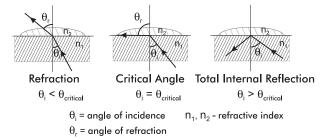
In the MA886 refractometer, light from an LED passes through a prism in contact with the sample. An image sensor determines the critical angle at which the light is no longer refracted through the sample.
