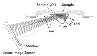
In the MA888 refractometer, light from an LED passes through a prism in contact with the sample. An image sensor determines the critical angle at which the light is no longer refracted through the sample. Specialized algorithms then apply temperature compensation to the measurement and convert the refractive index to: % Volume or Freezing Point.
