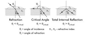
The critical angle can be used to easily calculate the refractive index according to the equation:
