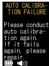
**CAUSE** Automatic calibration is not performed correctly.
