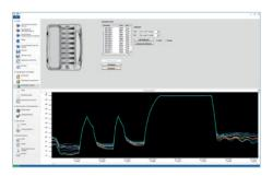
The data loggers are configured and read out using the testo 191 professional software. And all without needing a 400-page instruction manual and complicated menus. But using guided processes, helpful data visualization and the innovative 1-click report: the report recalls the parameters of the last measurement, so that you can meet your duty to provide documentation quickly and efficiently, without needing to reset all the report parameters time and again.
