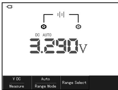
Picture 5-5 DC Voltage Measurement
