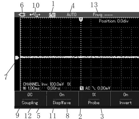
Picture 4-1 Instruction Picture of Display Interface Apart from the waveform, the display will display some detailed information about waveform and oscilloscope control setting.
