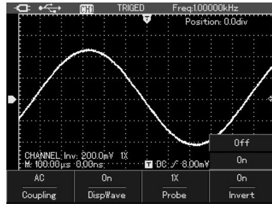
Picture 4-23 opposite phase display of waveform
