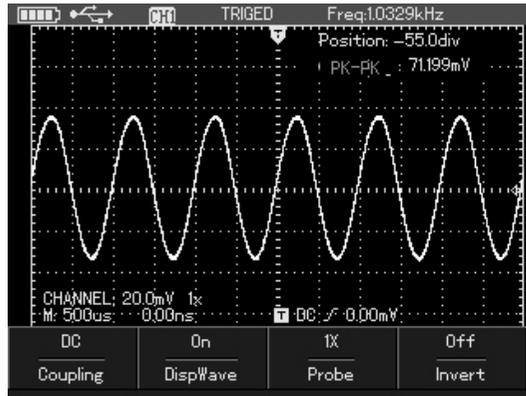
Picture 4-24 Setting the Signal with DC Bias
