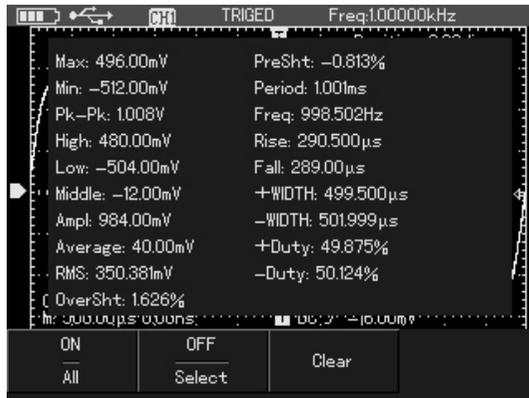
Picture 4-17 Measurement of All Parameters
