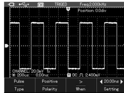
Picture 6-10 Trigger-Pulse Width Trigger
