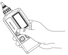
b. After the entire screen displays for 1 second, the default state is acceleration mode, if on the LCD displays the symbol  $\Box$  or  $\Box$ , please promptly replace the battery, as shown in following figure:
