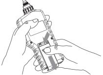
b. Insert a 9V battery into battery compartment, note the battery polarity, and then close the battery door, as shown in following figure:
