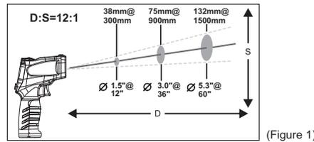
1. When taking measurement, pay attention to the Distance to Spot Size. As the Distance (D) from the target surface increases, the spot size (S) of the area measured by the unit becomes larger. The Distance to Spot size of the unit is 12:1. (Figure 1)
