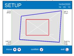
The calibration report has been designed to provide the user with an immediate view of the calibration conditions, in fact, the closer the blue rectangle (actual calibration data) is to the outside of the graph, the closer to ideality is the calibration and electrode conditions; vice versa, the condition worsens if the red rectangle is closer, which represents the limit of acceptability recommended by the supplier.
