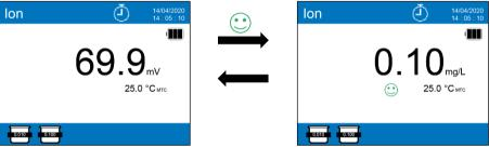
**Important**: If the device is not calibrated in reading mode, only the mV are displayed.
