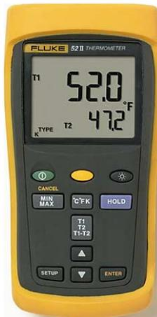
*Fluke 52 Dual Input Digital Thermometer*
