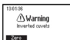
**Inverted cuvettes:** The sample and the zero cuvettes are inverted.
