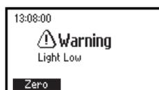
**Light Low:** The instrument cannot adjust the light level. Please check that the sample does not contain any debris.
