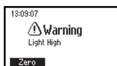
**Light High:** There is too much light to perform a measurement. Please check the preparation of the zero cuvette.
