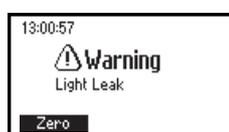
**Light Leak:** There is an excess amount of ambient light reaching the detector.
