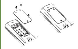
Replace the three 1.5V AAA alkaline batteries located in the battery compartment, observing the indicated polarity.
