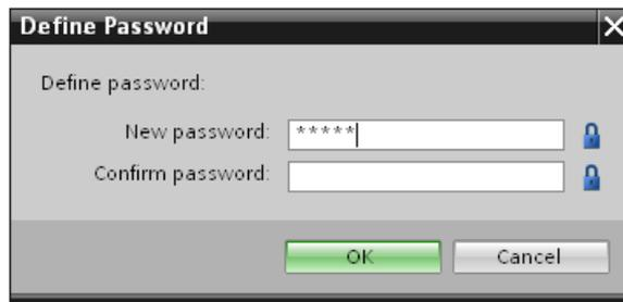
5. Enter the new password in the "New password" field. Enter the same password in the "Confirm password" field.
