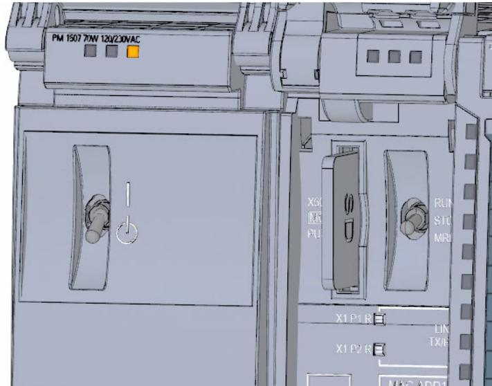
4. Move the switch for the load current supply (PM) to the position RUN.
