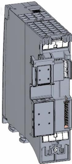
5. Mount the CPU on the mounting rail and screw tight.
