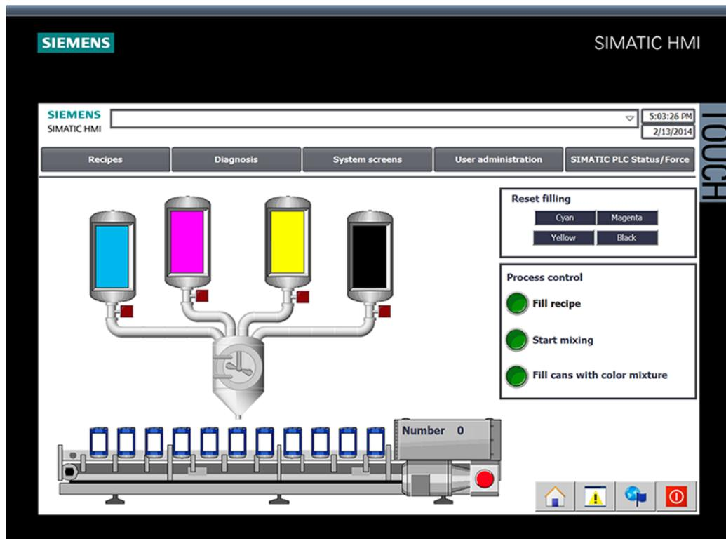
A connection to the CPU is established and the color mixing system is displayed in the simulation.
