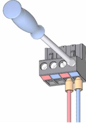
2. Wire the 4-pin connector plug with the 4-pin mains connection plug of the CPU.
