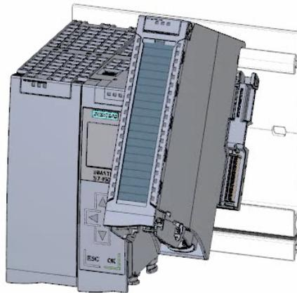
8. Attach the digital output module to the mounting rail and screw tight.
