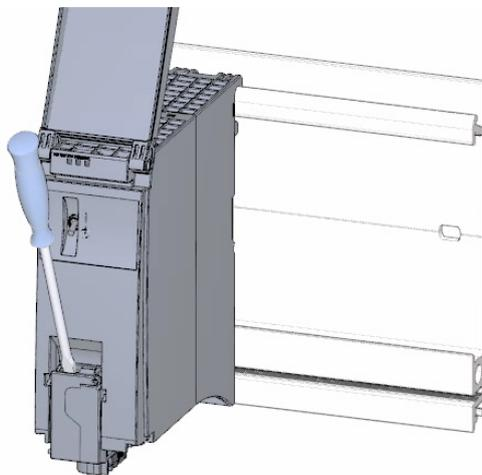
3. Remove the 4-pole connection plug and screw the load current supply (PM) tight.
