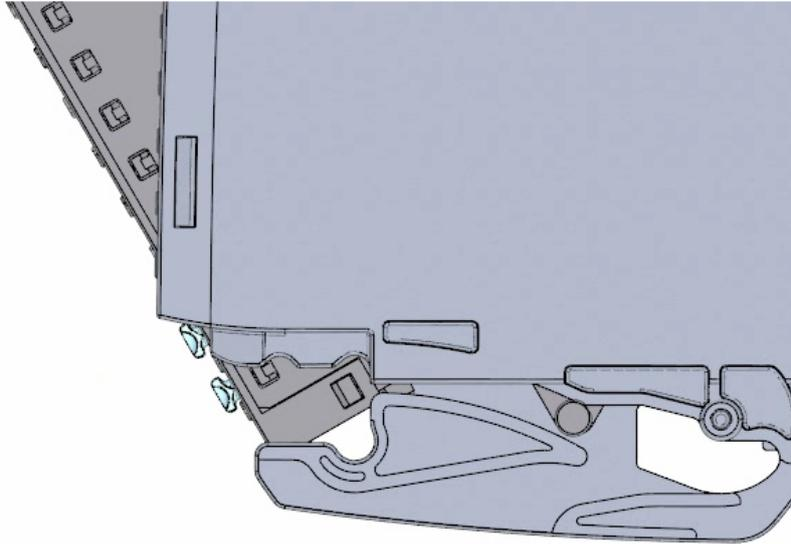
4. **Tip:** Pre-wired front connectors, e.g. for replacing modules, can be inserted directly.
