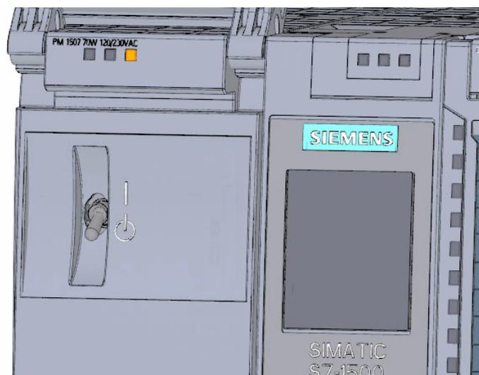
3. Insert a blank SIMATIC memory card into the CPU.
