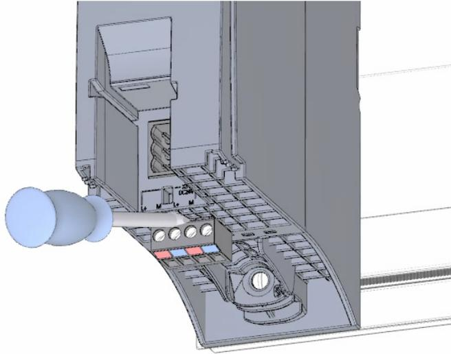
4. Insert the U-connector into the back of the CPU.
