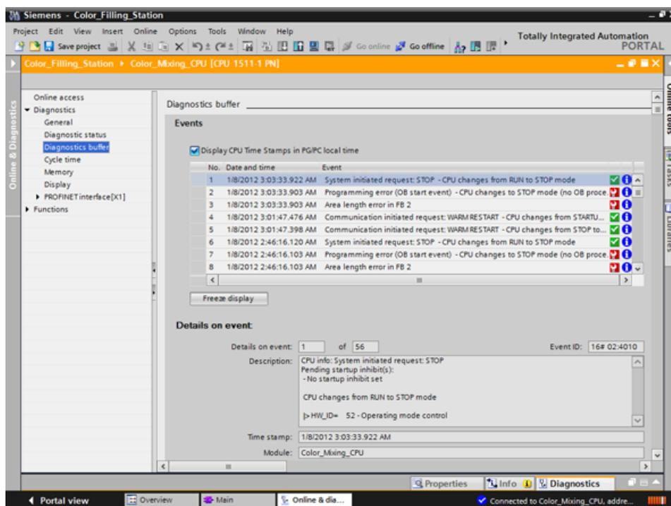
You can precisely evaluate the information and, for example, program the error handling in the block with STL/FBD/LAD and SCL programs. The block generates an error ID that is evaluated by the "GET\_ERROR\_ID" instruction. You can call the "GET\_ERROR\_ID" instruction in both the MAIN block and in the function blocks. The CPU remains in RUN mode.
