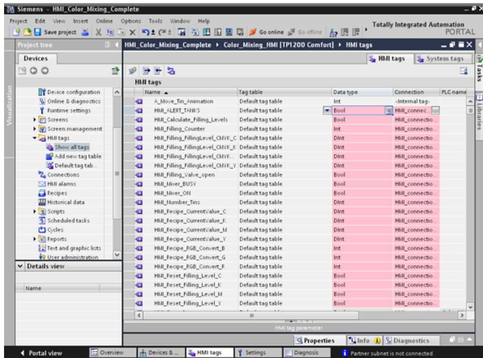
2. Select the HMI connection you have just configured in the "Connections" column.
