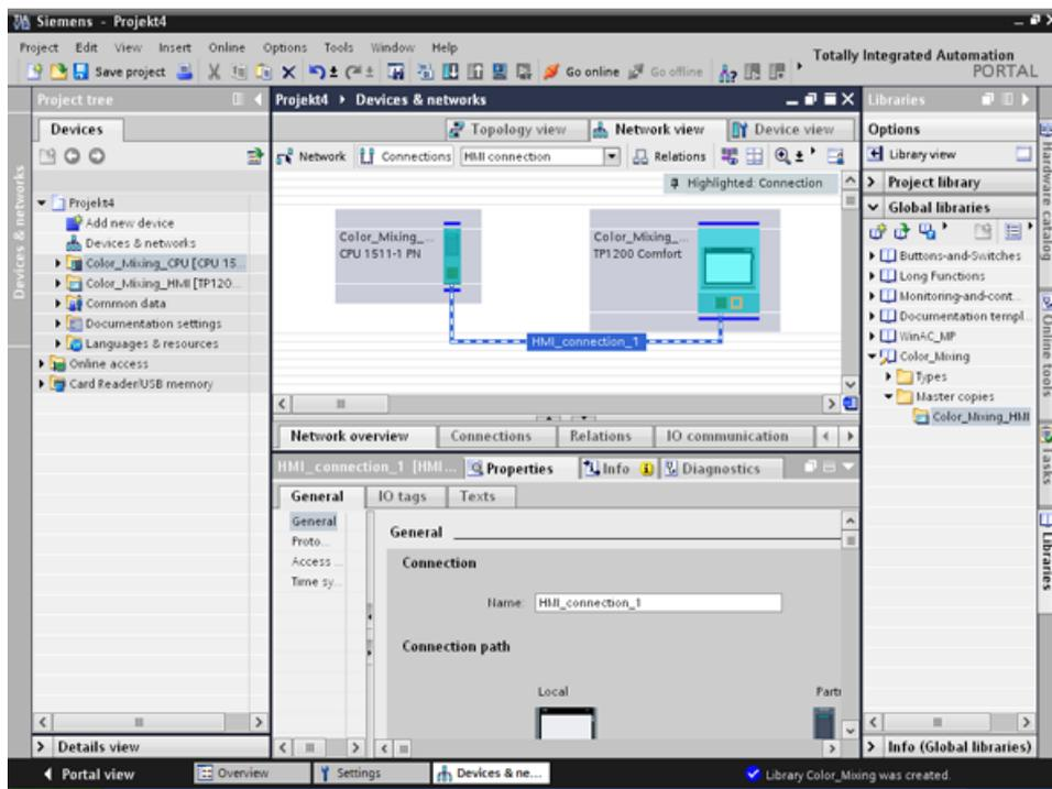
3. Click the communication partners in the "Network view" and change the PROFINET parameters in the Inspector window according to the requirements of your project.
