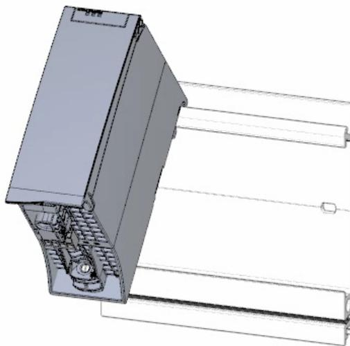
2. Open the front cover and pull out the mains connection plug.
