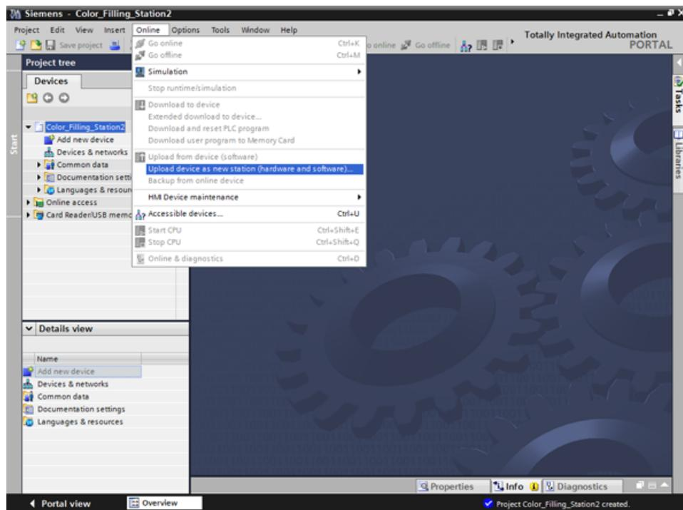
2. Select the interface with which the programming device is connected to the CPU. The search for accessible nodes starts automatically.
