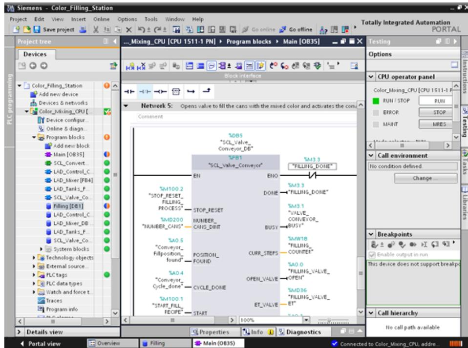
8. Open the "Date & time" folder from the "Instructions" tab and insert the "RD\_Loc\_T" block in the "Main" program block.
