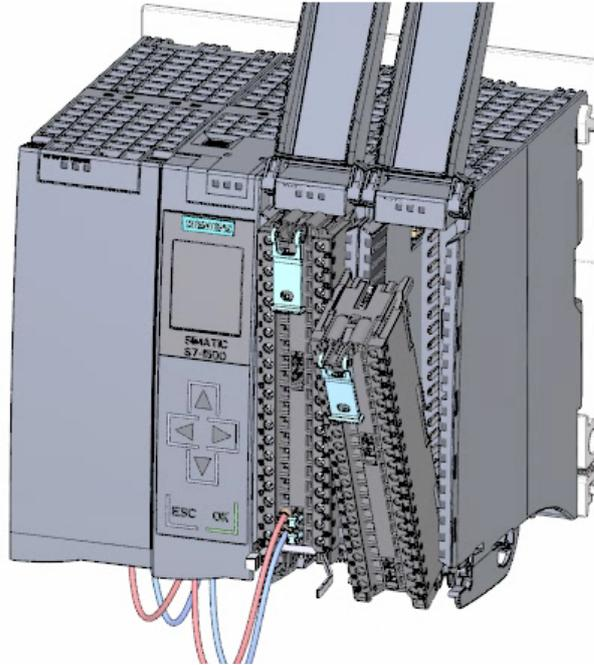
2. Use terminals 40 (M) and 39 (L+) from the digital input module to feed the supply voltage DC 24 V from the digital input module to terminals 20 (M) and 19 (L+).
