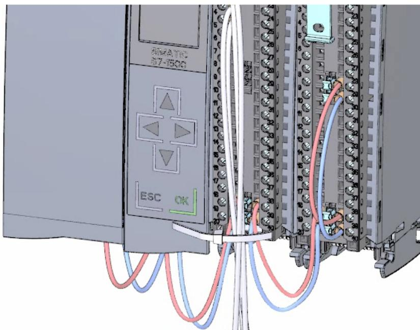
3. Move the front connector from the pre-wiring position to its final position. By doing this, you create an electrical connection between the front connector and the module.
