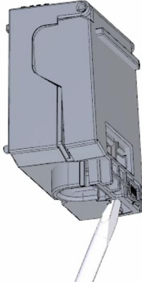
2. Connect the mains cable in the plug according to the connection diagram. You will find information on which voltage the plug is approved for on the side of the plug. You select the voltage by inserting the coding element accordingly on the back of the plug.
