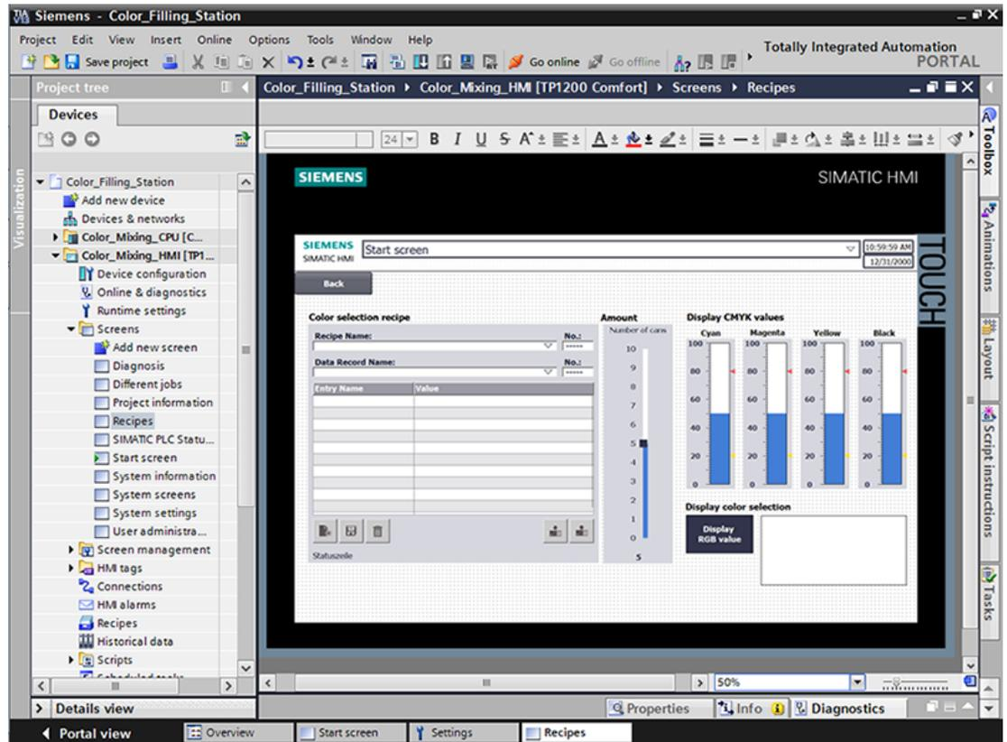
The color mixing system can produce the mixed colors "Orange", "Amber", "Green" and "Red".
