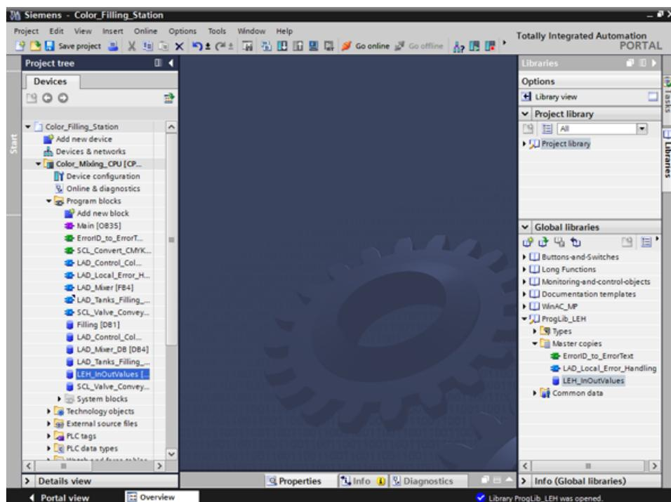
3. Call the "LAD\_Local\_Error\_Handling" function block in an empty network of the "Main" block.
