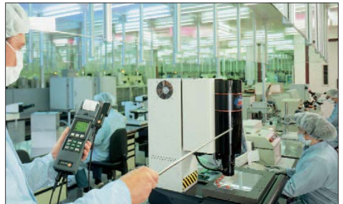
Checking the flow speed using the hot wire probe Part no.: 0635 1041
